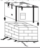
**8. COLLAPSE:** Unfasten all straps, separate inside and outside liners and push side hinges inward to collapse.
