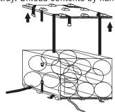
**7. FORKLIFT UNLOADING:** Unfasten 2" corner straps and unload cargo with forklift by releasing bottom tray 1.5" liner straps and lifting liners and top tray up and away from cargo.
