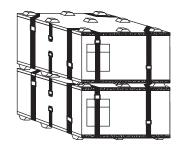
**6. TOP UNLOADING:** Unfasten 2" corner straps and unload MulePAC from the top by releasing top tray 1.5" liner straps and removing top tray. Unload contents by hand.
