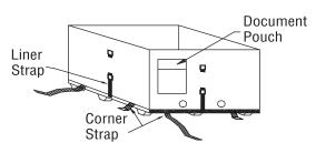
**3. WATER BAG:** Use Standard Potable Water Procedures for cleaning Water Bag Prior to use. Place 10mm plastic protective sheet on tray deck. Place clean empty water bag on top of protective sheet with 3/4" outlet valves aligned with 2 liner holes on front (Document Pouch) side, with 6" inlet cap facing up, and with the 4 bag corners aligned with the box corners.
