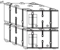
**7. COLLAPSE WATERBOX:** Unfasten all straps, remove top tray, separate inside and outside liners and push side hinges inward to collapse.
