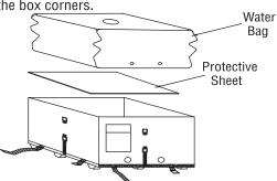
**4. Fill:** Close outlet valves, remove inlet cap and begin filling with Potable Water. While filling (first 1-2" of water) insure the bag corners are aligned with the box corners and the bag bottom wrinkles are removed.
